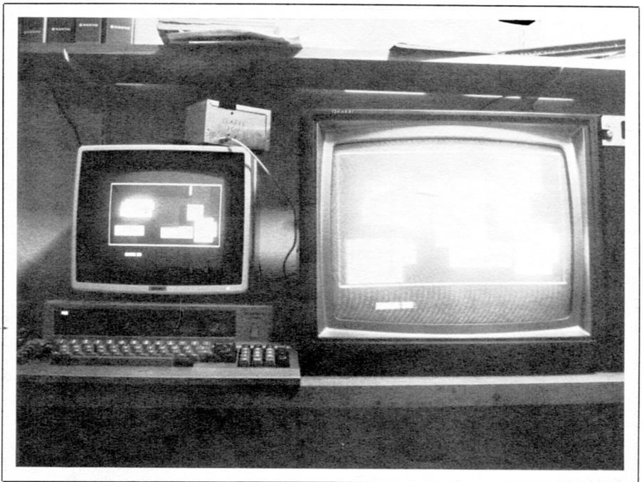
FIGURE 2: The same graphic image is shown on a Sanyo 555 12-inch green monitor and a 19-inch color TV. What appear as darkly shaded rectangles on the green monitor appear as brightly colored rectangles on the TV.
